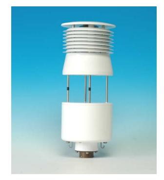
Designed for maximum portability and utility, the AIO Weather Sensor is uniquely applicable for rapid deployment and use by one person under all conditions. The unit may be mounted on a tripod or vehicle mast.
