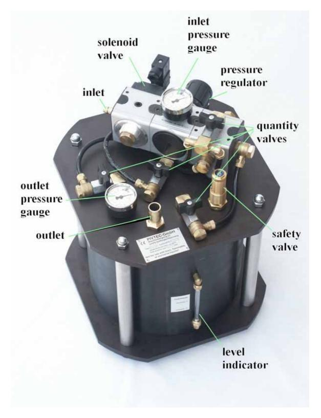
Figure 5: The PivPart45-M particle generator
