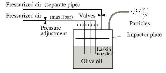
Figure 1: Principle of the PivPart45 particle generator
